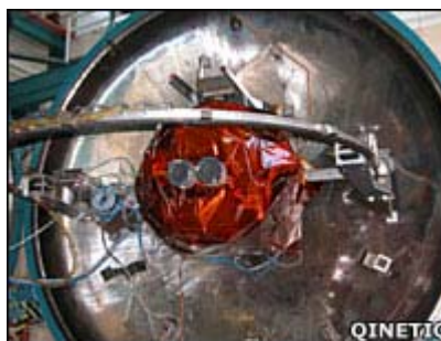
QinetiQ's engine assembly about to go into a vacuum test chamber
